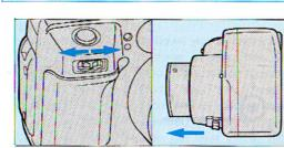
Looking through the viewfinder, aim the camera at your subject. Then, use the zoom control, located in front of the shutter-release button, to adjust the perspective as you like. Sliding the zoom control to the left decreases the focal length and moving it to the right increases the focal length. The focal length setting can be checked by referring to the zoomposition indicator in the data panel.
