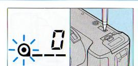
After the last frame on the roll is exposed, film rewind starts automatically. When rewind is complete, the frame counter returns to 0 and the data panel's film-cartridge symbol blinks to indicate that the film can be removed. Open the back cover and remove the film.
