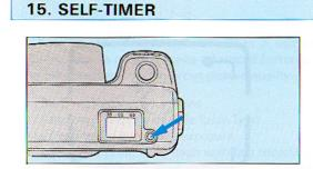
To set a ten-second shutter release delay, press the self-timer button to select self-timer mode. The self-timer indicator (\*) will appear in the data panel. To start the self-timer, aim the camera in the usual way and press the shutter-release button all the way down. During the countdown to exposure the selftimer light, located on the front of the camera, blinks to indicate operation.
