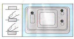
In describing camera operation, this manual refers to two shutter-release button operating positions: a pre-release, "partway down" position, which activates the eyepiece-indicator lamps, and an "all-theway" down position which actually release the shutter. Both operating positions of the shutter-release button, as well as its rest position, are illustrated.
